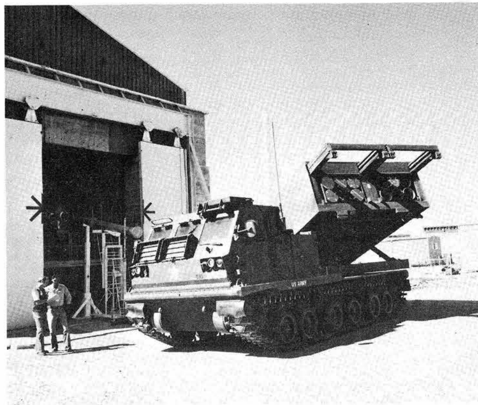
OUTDOOR TESTING of very large devices, including rocket launcher above, is now possible with the Hermes II facility. This new mode transports the Hermes II beam along a drift tube to a point outside the building where the beam pulse is converted into bremsstrahlung radiation.
